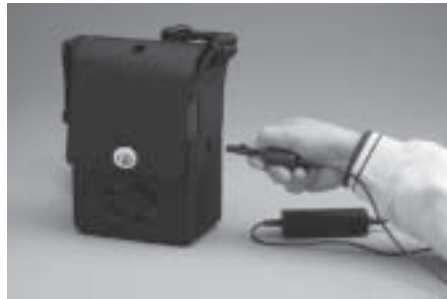
Figure 5: Internal Battery Charging
